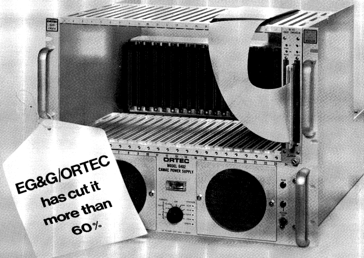
Our basic CAMAC system: crate, power supply, DC-011, unibus extension cable.
